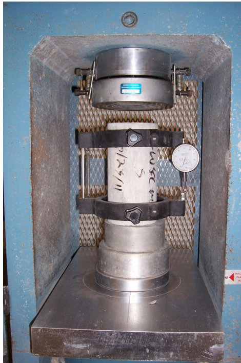
Figure 3.11 Modulus of Elasticity Apparatus
