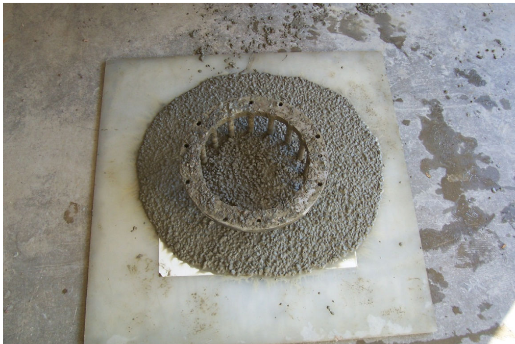
Figure 3.10 J-Ring Test Part 2: Measure the Flow
