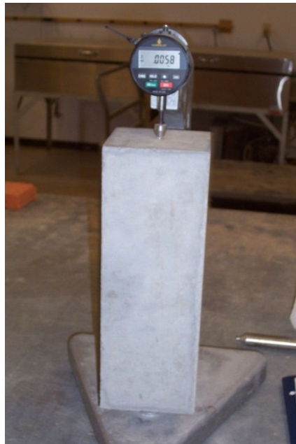
Figure 3.12 Prism Resting in Shrinkage Apparatus
